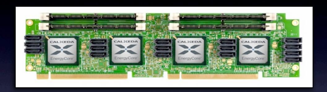
"The EnergyCore is a single chip with a Cortex-A9 ARM processor running between I.IGHz and I.4GHz. The chip includes 4MB of cache, an 80-Gigabit fabric switch and a management engine for power optimization. Servers with the chip, 4GB of memory and a large-capacity solid-state drive [SATA] draw 5 watts of power. Besides using a low-power ARM processor, Calxeda has cut down chip power consumption by integrating key server components."
