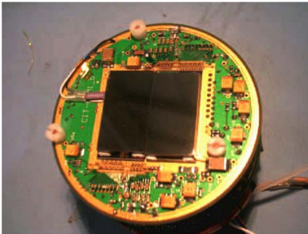
Fig. 2 Photo showing a HEFT focal plane detector system. Two CdZnTe/ASIC hybrid pixel sensors are mounted side-by-side
