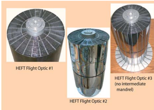
Fig. 1 Photo of the three HEFT flight optics. Each unit is fabricated from formed, multilayer-coated glass
