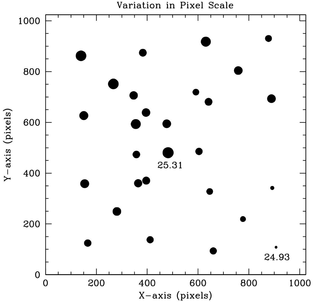
Fig. 1.— Positional dependence of the pixel scale for the night of Jun 23, 2002 (from Memo I). The binary WDC 18055+0230 was observed at angle of  $63.5^\circ$ . The point size indicates the pixel scale, decreasing linearly from the largest value (25.31 mas/pix) to the smallest one (24.93 mas/pix).
