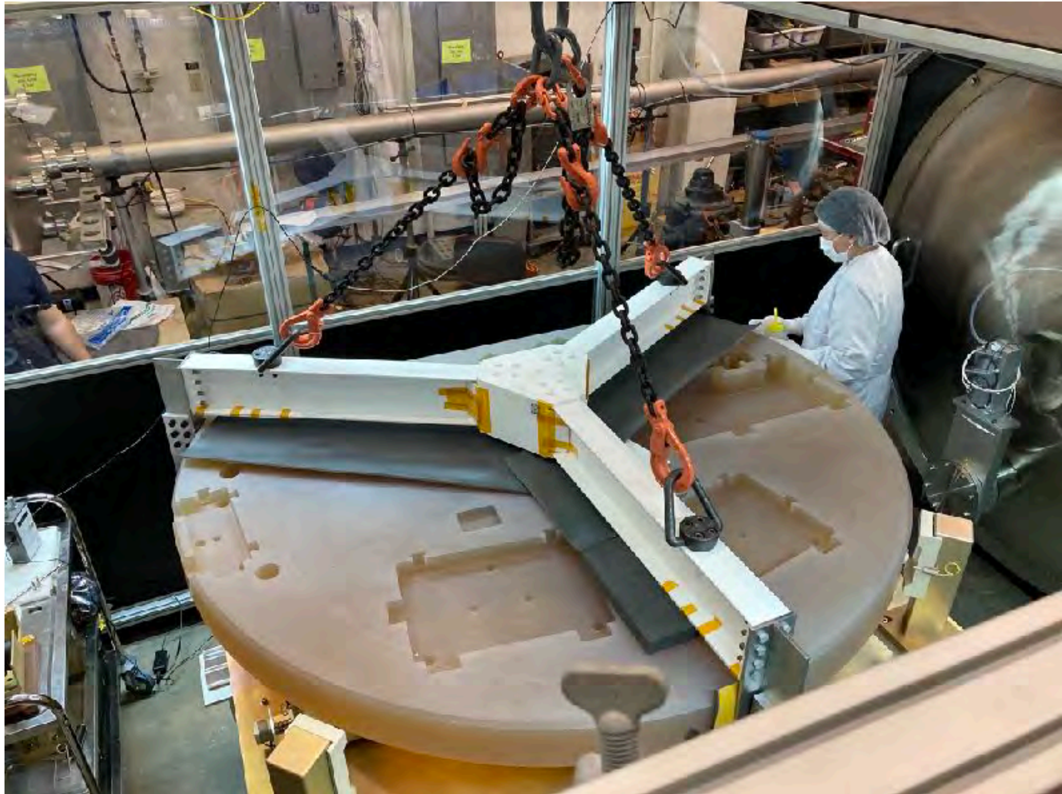
Spectrometer optical bench being lifted onto isolation frame
