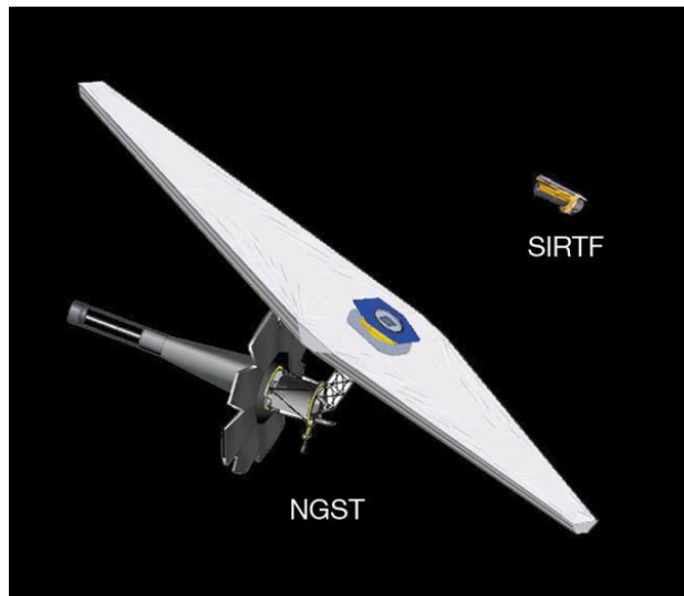
Figure 4. Evolution of infrared space telescopes. Shown to relative scale are SIRTF, a 0.85 m cryogenic telescope to be launched in 2002, and a concept for the 8 m NGST. Both will orbit far from the Earth, with thermal shields on the Sunward side.
