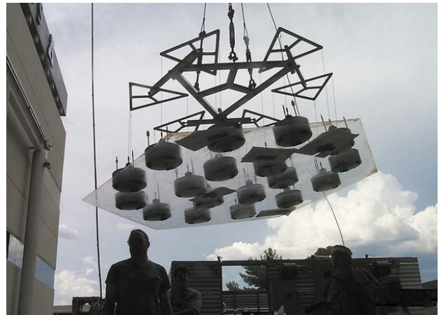
Figure 5. A 2 m hexagonal concave glass mirror is lifted clear after separation from the support on which it was thinned and polished. It is 2 mm thick and weighs just 30 lb (13.6 kg). (Image courtesy of J. Burge.)
