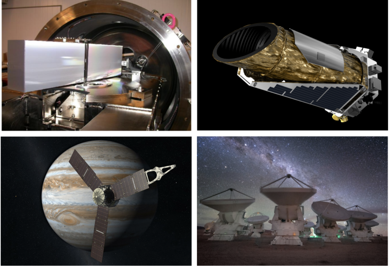
Figure 1: Observational facilities yielding key constraints for planet formation theory. Top left: the H RPS spectrograph (Mayor et al. 2003) installed at ESO’s 3.6 Meter telescope in Chile. Through its unprecedented radial velocity precision of 1 m/s, it allowed for the first time the discovery of low-mass extrasolar planets and the study of exoplanetary system architectures in the mass-distance diagram. Top right: the N S Kepler satellite (Borucki et al. 2010). With ultra-precise transit photometry it has unveiled the demographics of the transiting exoplanet population. Bottom left: The N S Juno satellite in orbit around Jupiter has deeply changed our picture of the interior of giant planets. Bottom right: the joint American-European-Japanese Atacama Large Millimeter/Submillimeter Array (ALMA) has started a new era in the study of protostellar and protoplanetary disks, the cradles of planets (Image credits: H RPS: ESO; ALMA : CC BY 4.0 ESO/Beletsky; Kepler: N S ; Juno: N S /JPL-Caltech)
