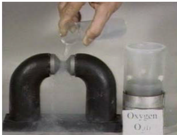
Figure 5. Demonstration showing blue liquid O_2 attracted to the poles of a permanent magnet. From http://jchemed.chem.wisc.edu/jcesoft/cca/CCA2/STHTM/PARANIO/9.HTM
