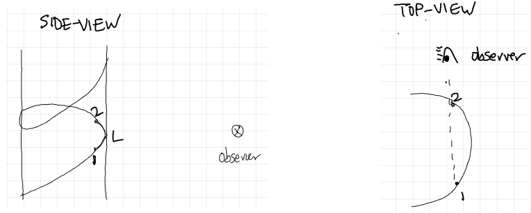
Figure 2 The helical trajectory of a relativistic electron in a magnetic field (along the vertical axis).
