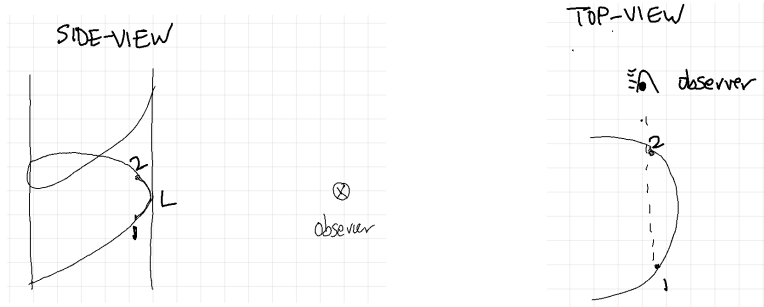
Figure 1: The helical trajectory of a relativistic electron in a magnetic field (along the vertical axis).
