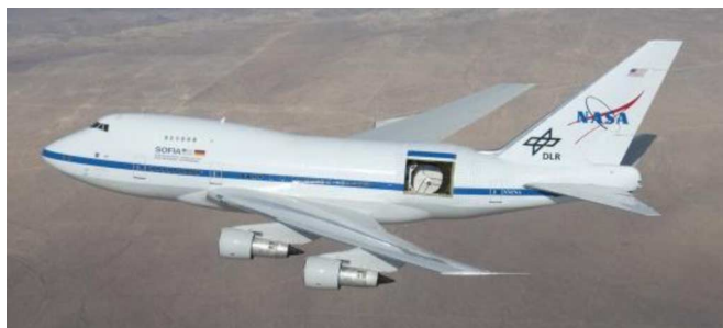
Fig. 13. SOFIA is a Boeing 747 SP modified to carry an open port 2.7 m telescope (chopped aperture 2.5 m), that enables routine access to the highest THz frequencies [90].
