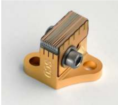
QCW – Quasi Continuous Wave 60 to 480 watts @ 56A
