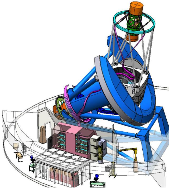
Figure 3.2: The *Dark Energy Spectroscopic Instrument* (DESI) is a massively-multiplexed spectrograph with 5000 spectroscopic channels. This amazing spectrograph will be mounted at the prime focus of the Kitt Peak Mayall 4-m telescope and expected to start operating in 2019. While the primary purpose is cosmography the instrument has the ability to accelerate time domain astronomy by pre- or post-observations of host galaxies of cosmic explosions.
