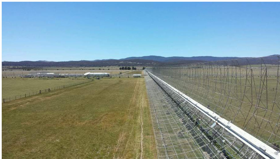
View of the Molonglo valley site near Hoskinstown, NSW, Australia, showing the UTMOST telescope reflector surface and feed line.
