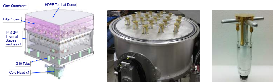
Figure 3: [Left]: Cutaway schematic of ALPACA cryostat showing inner structure of the top-hat dome and Rohacell foam layers. [Center]: Successfully tested (at Arecibo) AO-19 cryo-PAF without three foam layers and HDPE top-hat dome. [Right]: Dipole/LNA re-insertable package, each cylinder contains two LNAs. The press fit connectors are at its base.
