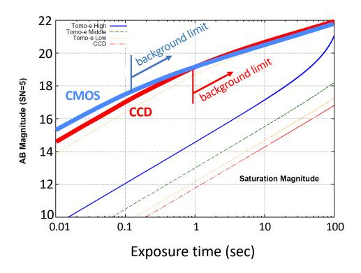
CMOS: efficiency=0.65,  $N_{read}$ =2 e-CCD: efficiency=0.90,  $N_{read}$ =5 e-
