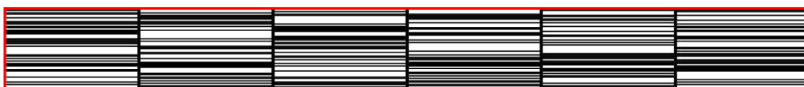
Figure 6.5 : The coded mask plate with six different mask pattern used in each of the three SSM cameras.
