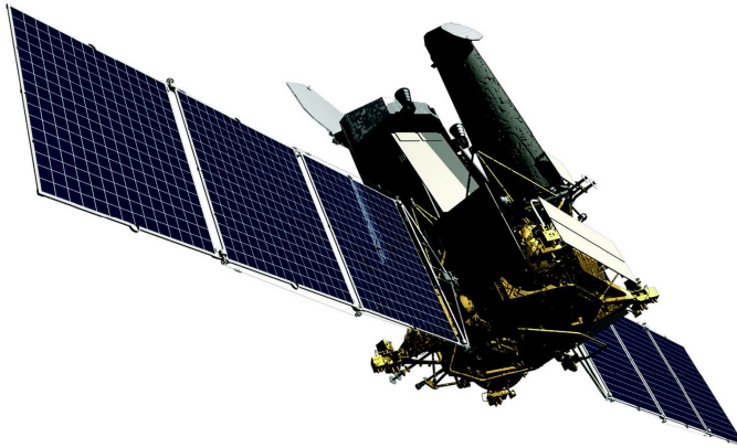
Figure 11.1. The SRG spacecraft is based on the “Navigator” multiuse bus of the NPO Lavochkin Scientific Production Association, Khimki, Russia. The spacecraft is three-axis stabilized and has an estimated launch mass of ~2712.5 kg (total payload mass of 1165 kg). (Reproduced courtesy of Roscosmos TV.)
