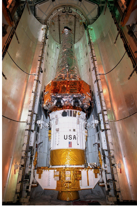
Figure 0.7. The Chandra X-ray Observatory in Columbia 's cargo bay. The IUS is marked by the letters "USA." (Courtesy of NASA.)
