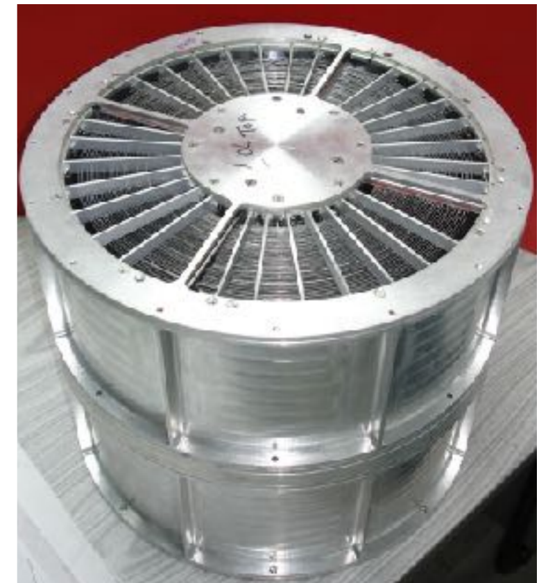
Mirrors: Nested & Segmented conical surfaces in Wolter type I geometry working at Grazing incidence 39 nested shells
