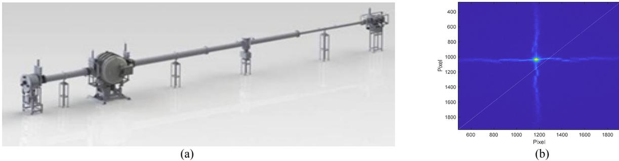
Figure 10: (a) X-ray imaging beam line (b) X-ray image captured by GSENSE400BSI.
