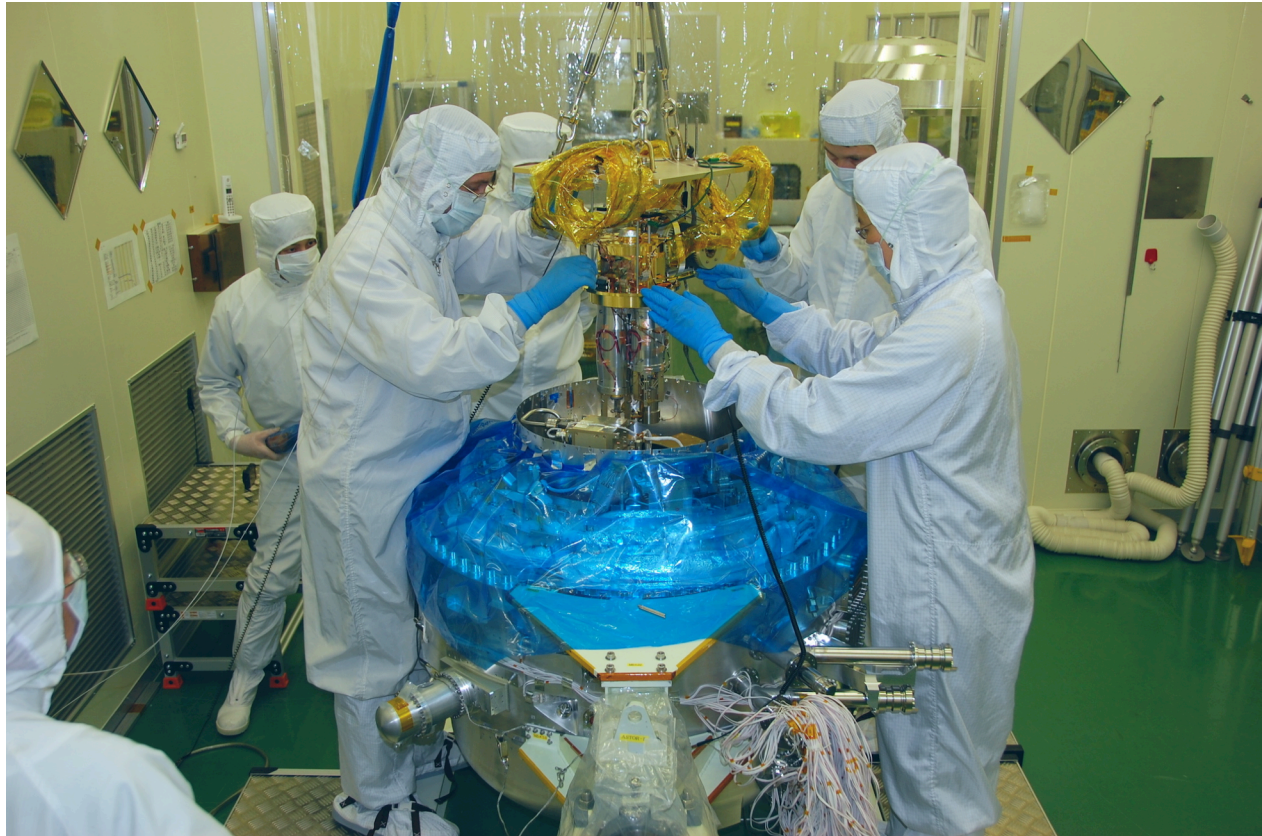
Fig. 4 The integrated SXS detector and ADR assembly being installed into the flight dewar in March 2014 at Sumitomo Heavy Industries, Japan.
