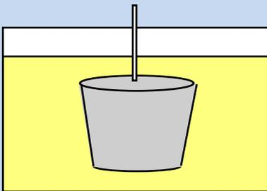
7. Electroform Nickel/Cobalt shell onto mandrel
