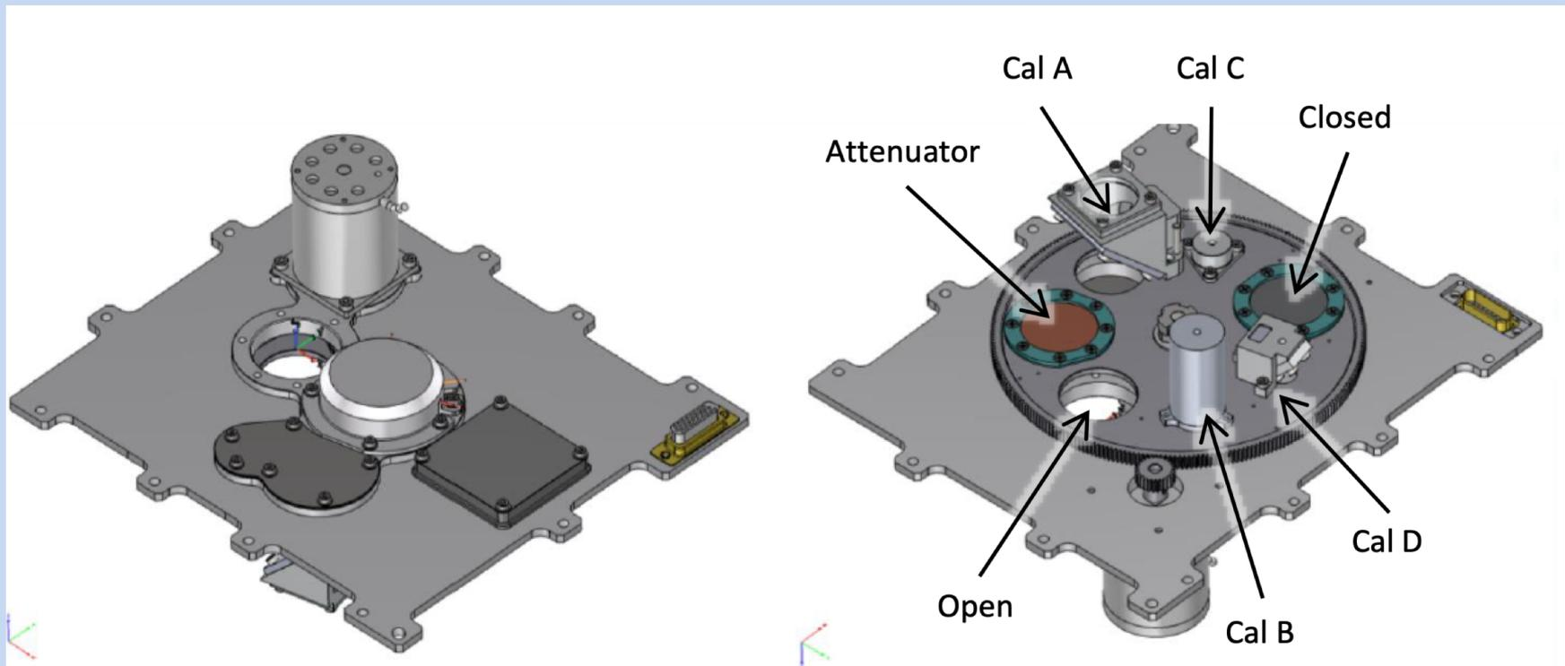
Filter and Calibration Wheel (FCW), providing open, attenuator, and closed positions, plus four  $^{55}\text{Fe}$ -powered calibration sources:
