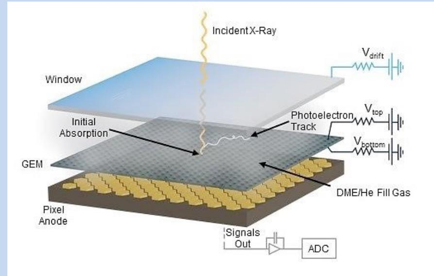
The distribution of the photoelectron initial directions determines the degree of polarization and the position angle
