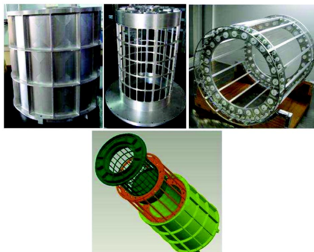
Fig. 4. Fabricated parts of the cylindrical detector and the total assembly
