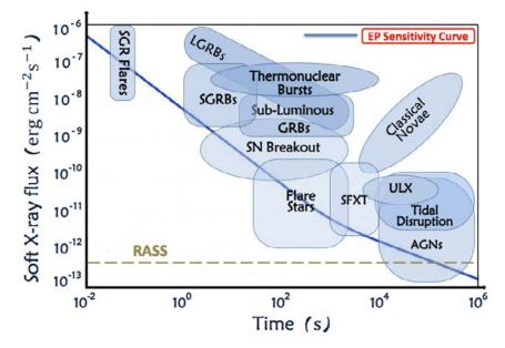
Fig. 15: Sensitivity of WXT as a function of exposure time.
