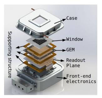
Fig. 19: Sketch of the focal-plane detector for a WXT module (credit: Hua Feng, Tsinghua University & NAOC).
