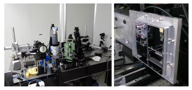
Fig. 17: Laser-guided MPO assembling and contactless online quality-monitoring system for the building of the EP/WXT. prototype module (below left). Currently an assembling precision of micro-meter or arc-second has been realized for a 2x2 MPO pieces array using a quasi-stress-free control system (below right) (credit: Chen Zhang, X-ray Imaging Lab, NAOC).
