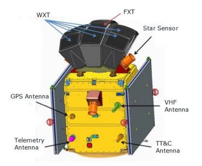
Fig. 16: Layout of the Einstein Probe satellite (courtesy of NAOC & MicroSat, CAS).
