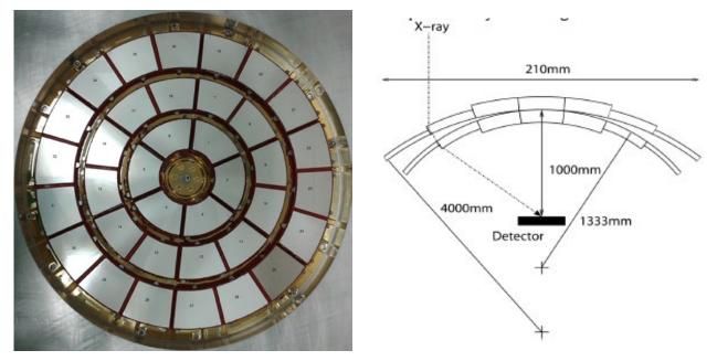
Fig. 10: Left: The MIXS-T aperture (credit: R. Willingale, the University of Leicester). Right: The curvature of the tandem plates (not to scale) (credit: Fraser et al. 2010 P&SS 58, 79).
