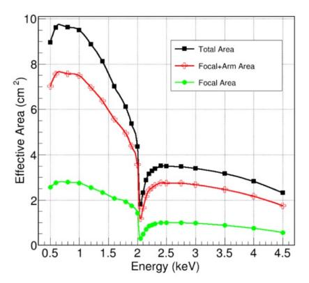
Fig. 14: Effective areas for WXT (results of simulations based on Geant4/ XRTG4; see Zhao, et al. Proc. SPIE 9144, Space Telescopes and Instrumentation 2014: Ultraviolet to Gamma Ray, 91444E; doi:10.1117 /12.2055434).
