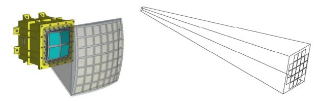
Fig. 11: Lobster eye telescopes. Left: wide field. Right: narrow field. (Credit: R. Willingale, University of Leicester)
